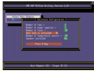
It is important to note that the enclosure has been programmed with the information on this screen and that information can be changed using the Firmware Option menu if a different setup is required. For example; If a power supply is removed, the enclosure configuration will still report that the number of power supplies is '2'.
